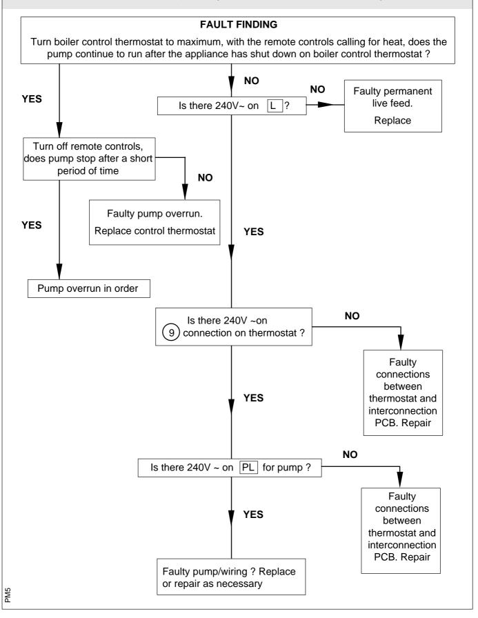
Before detailed checking of electrical components ensure that remote controls are calling for heat. Check that the gas supply is free of obstructions and purged of air. Check the overheat thermostat and fluehood thermostat have not operated. Isolate the electrical supply and physically check ALL cables, connections and the printed circuit board (PCB) fuse. Check the air tubes to air pressure switch.
