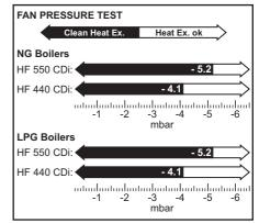
Pressure readings in the black area indicate that the heat exchanger requires cleaning.
